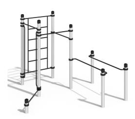
The complex consists of eight vertical columns of different height, four crossbars 1200 mm in length, a Swedish wall section, two climb-down bars 1932 mm in height and two parallel bars 1932 mm in length. The distance between the inside surfaces of the parallel bars is 550 mm. The height of the Swedish wall is 2073 mm, width - 1200 mm. The distance between the crossbars of the Swedish wall - 407 mm. The structure is secured together with siluminium clamps. Weight - 154.3 kg.
