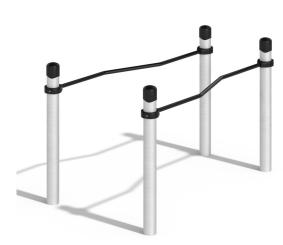
The complex consists of four vertical columns with 1200 mm height and two multi-width parallel bars 1790 mm in length. The distance between the parallel bars is 598 mm at one end and 1198 mm at the second end. Total width difference for the parallel bars is 600 mm. Construction is secured together with siluminium clamps.
