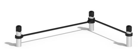
The structure consists of three vertical columns and two crossbars. The length of crossbars is 1200 mm and 1758 mm. The structure is secured together with siluminium clamps. Weight – 23.1 kg.
